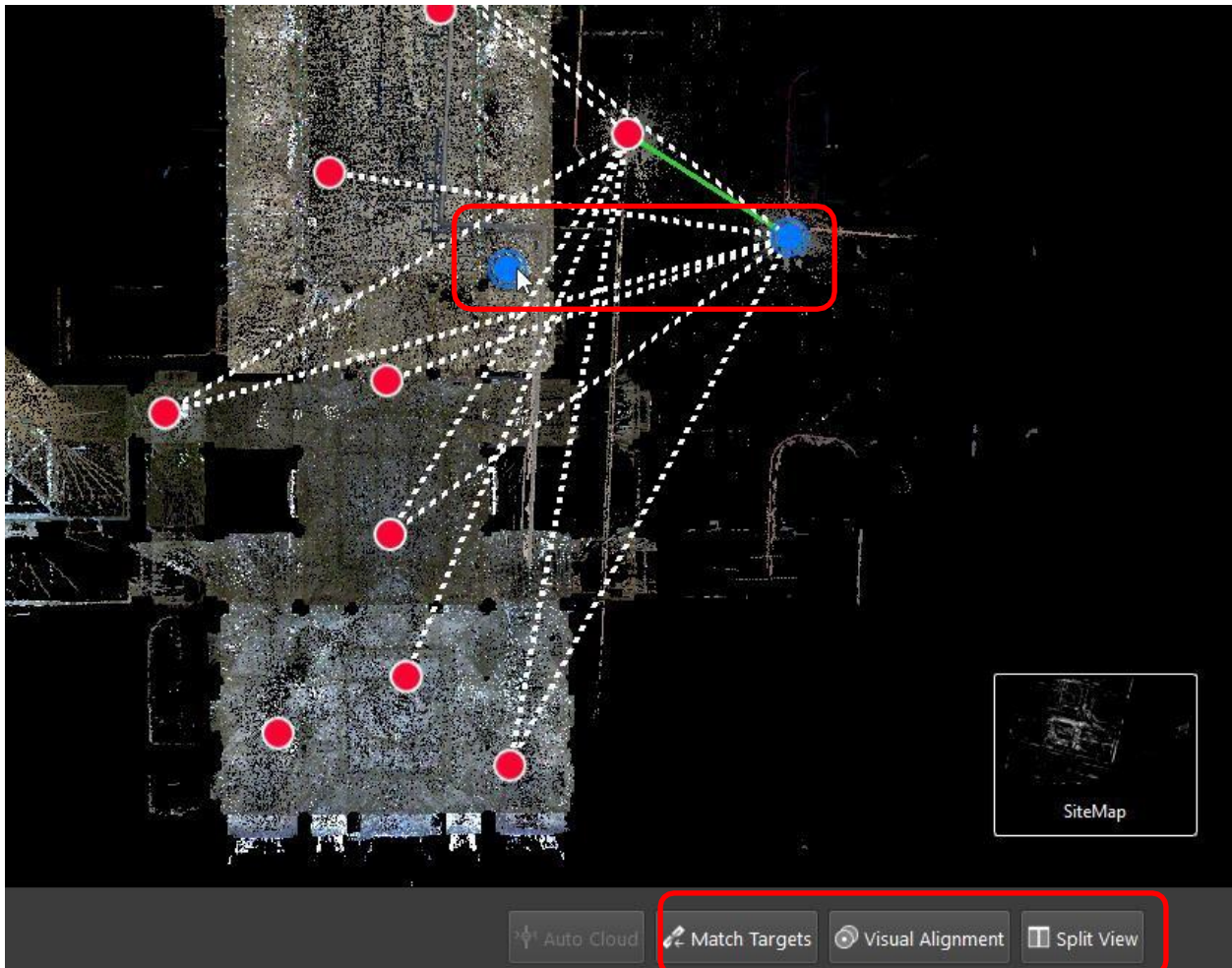
Two selected objects shown. One is a Setup and the other is a WayPoint. Once selected, various methods can be used to join the scans together.
